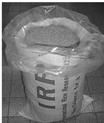
FIGURE 3.4. IRRI super bag (the gas- and moisture-proof liner)
