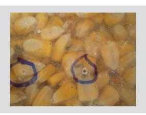
Figure 4. Holes in SuperGrain (GrainPro, Inc.) hermetic storage bags created by insects. Note the insects inside the bag feeding on the grain.
